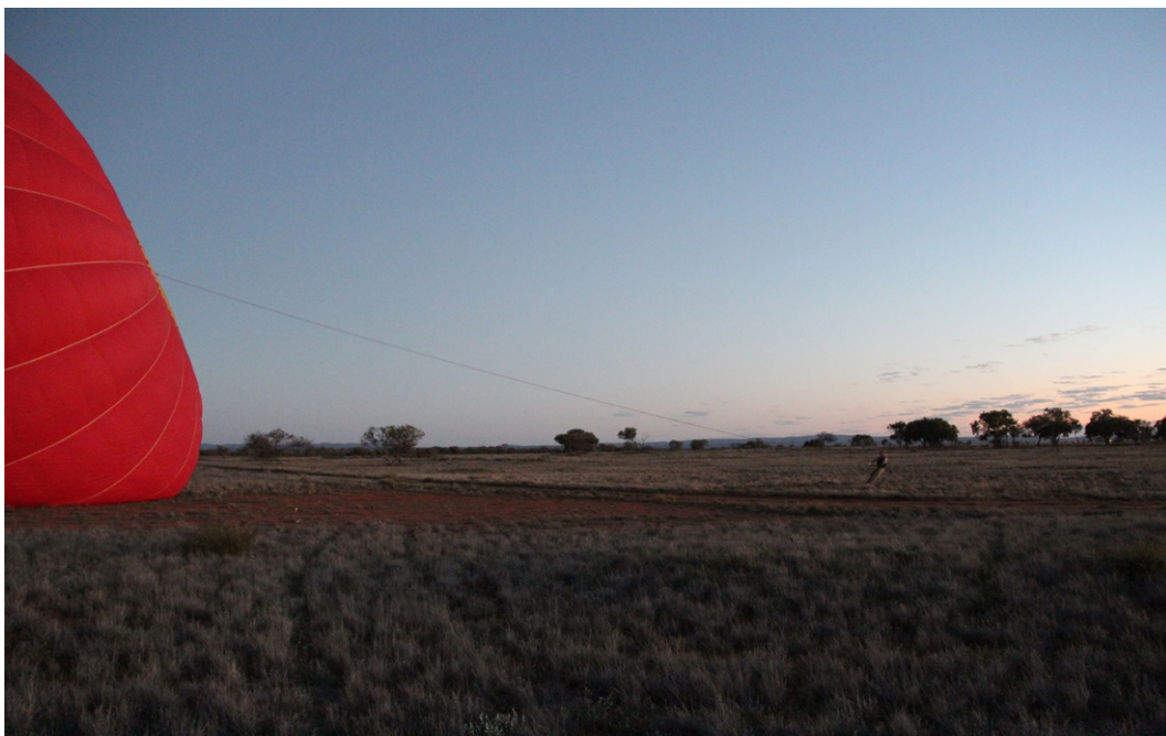
Example of a ground crew member controlling the balloon crown line. Source: Australian Transport Safety Bureau
